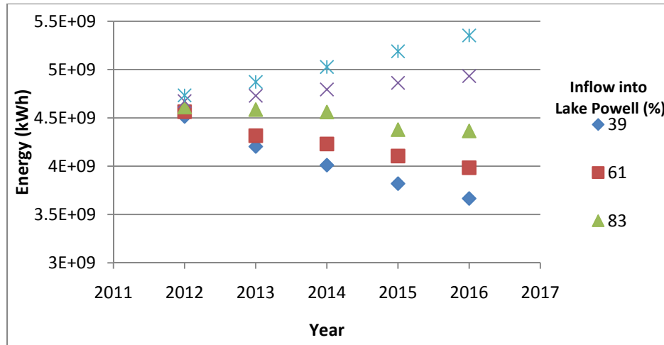
Figure 6- Effect of Inflow to Lake Powell on Power Generation at the Hoover Dam
